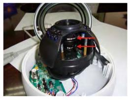
9. Top screw adjusts focus, bottom screw adjusts lens size.
